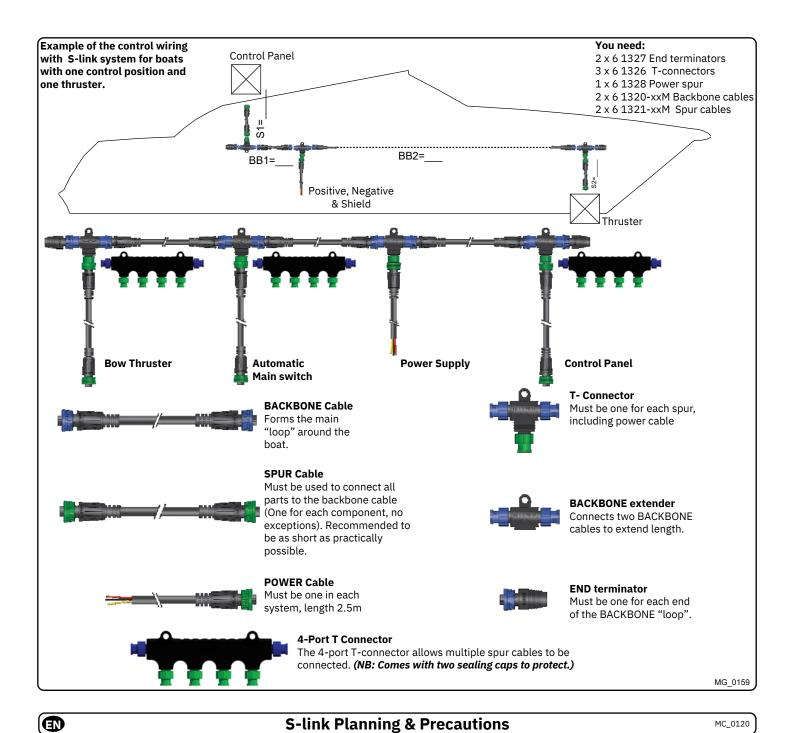
S-link is a "CAN" based control system with full intelligent communication between all units in the system. Main advantages include:
